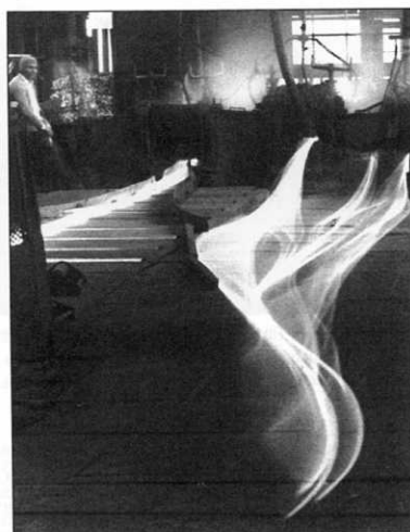
Red-hot bars passing through the mills at Birchley and snaking across the mill floor. (Terry Daniels collection)
