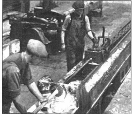
A draw-bench at Accles and Pollock with the 'drawer' feeding the tube through the die and the 'dogger' ensuring that the tag is firmly gripped. (Terry Daniels collection)
